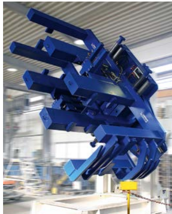
25T251W/099 - Inverter for steel sheets
